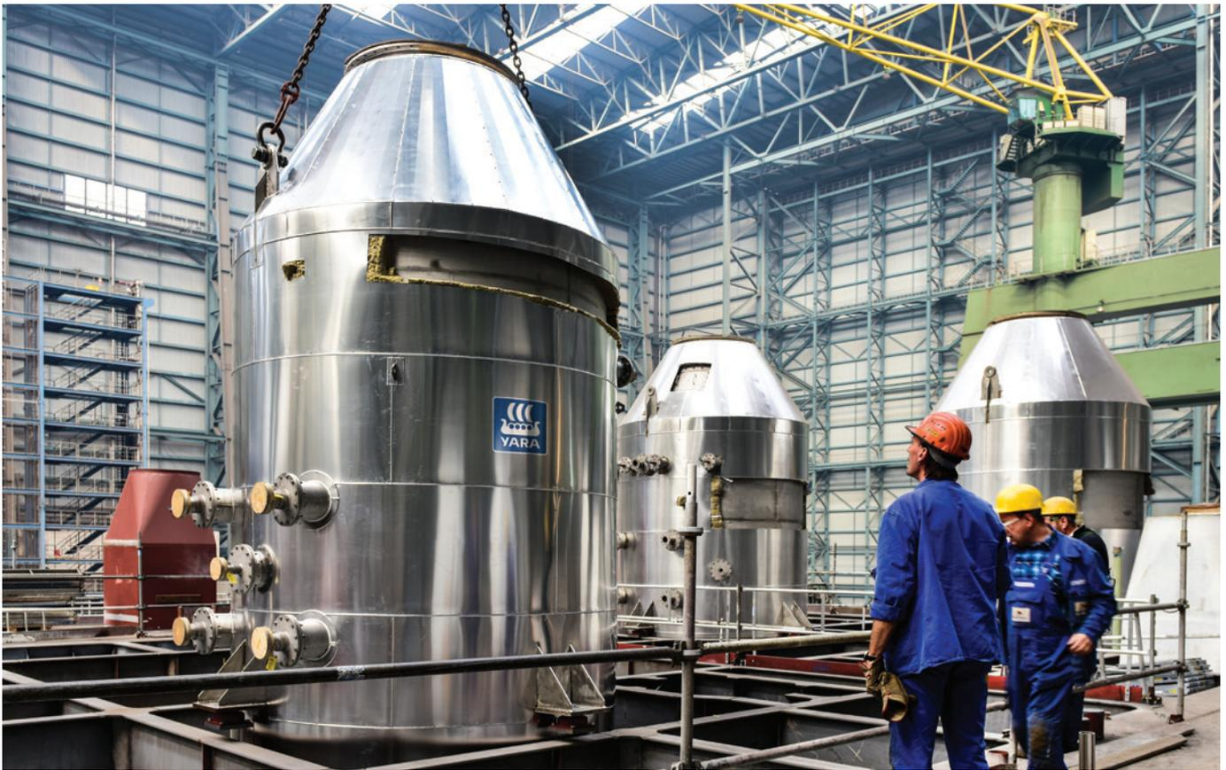
Closed loop scrubber systems are necessary for marine areas with low natural alkalinity. Once cleaned, effluent can be safely discharged into the water. When operating in a zero discharge region, the effluent must be collected in a holding tank for land-based disposal.
