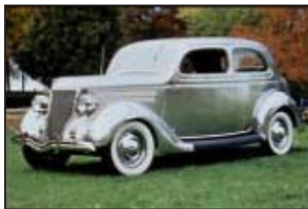
STAINLESS STEEL CAR. Built to last, but not very fuel efficient by today's standards.
