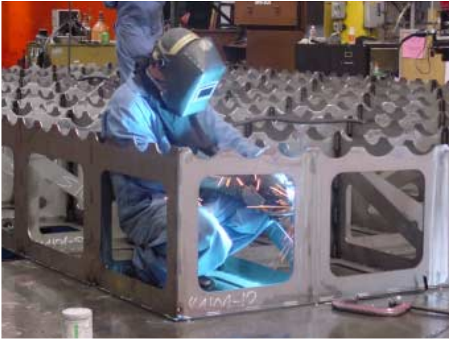
A WELDER pieces together the 'egg crate' base that will support the mold surface for the outer skin of the Airbus A380 wingboxes.
