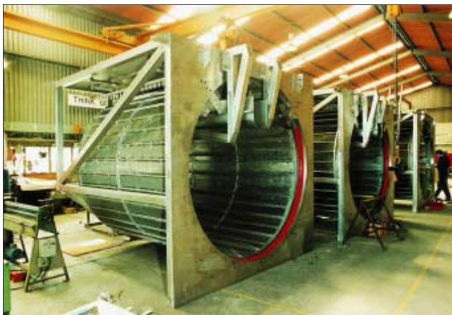
BOUND FOR CHINA: Three rotating drums, made of S31600 stainless steel, near completion in Auckland, New Zealand prior to being shipped to a waste water treatment plant in Shenzhen, China.
